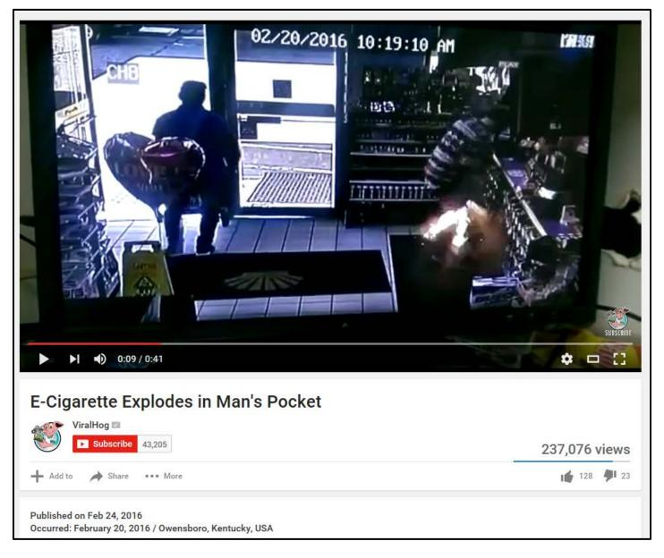
Screen shot of exploding lithium-ion battery in pocket of man's pants.
